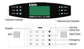
Alarm Panel back schematic diagram:
